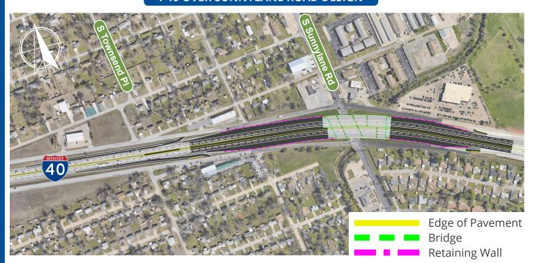
As part of the I-40 East Corridor improvements, ODOT has advanced plans to replace the existing eastbound and westbound bridges on I-40 over Sunnylane Road. These bridges are considered at risk of becoming structurally deficient. The new bridges will be longer and wider than the existing bridges to accommodate proposed future lanes on I-40 and Sunnylane Road. The Sunnylane project will replace the bridges only and will not add lanes to I-40 or change the existing frontage roads.
