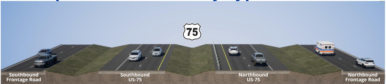
This image shows the future cross section of US-75 with two one-way parallel frontage roads.
